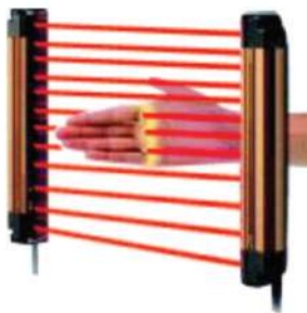
手掌检测用最小检测物 体光轴间隔20mm分辨率 Φ32mm The hand detecting type with axis spacing of 20mm and with 32mm resolution.
